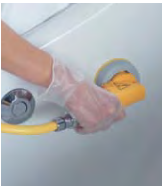
AIR SPA DISINFECTION: The air spa can be fully disinfected by flushing through with ARJO Cleaner/Disinfectant. This economical method reduces bacterial loads to a safe level.
